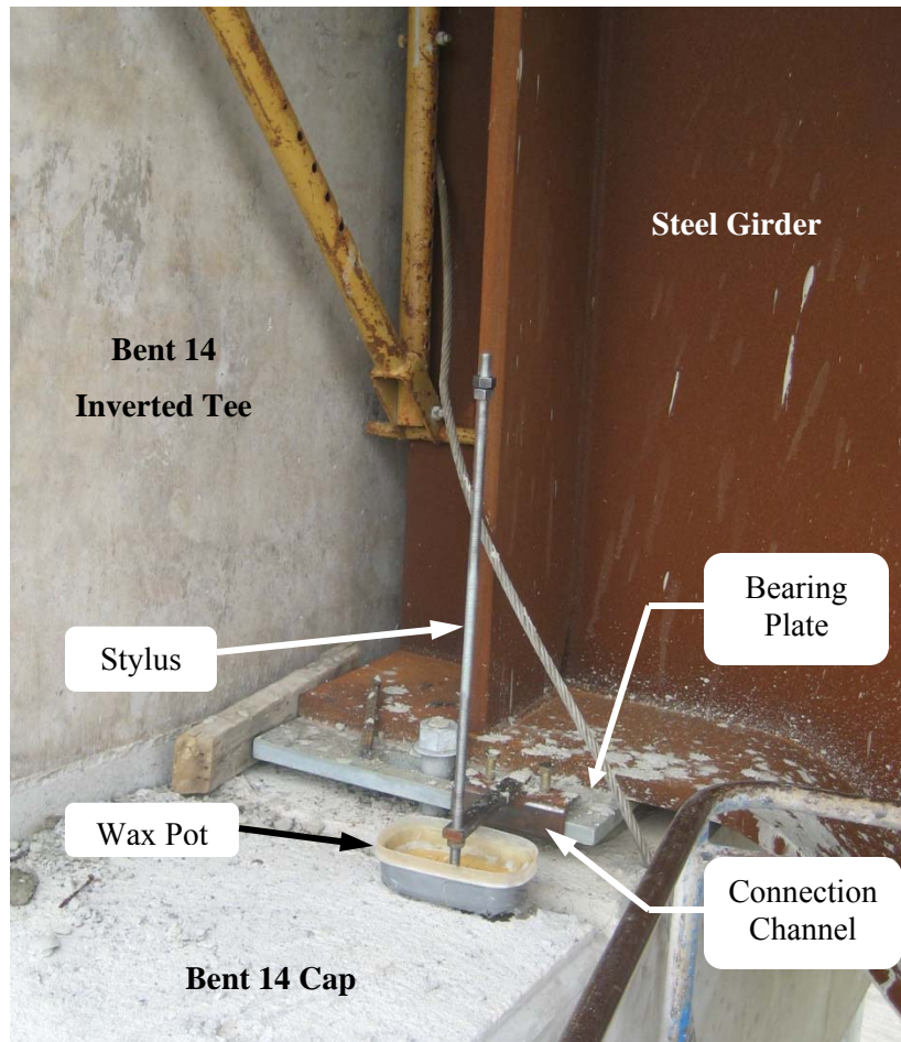
Figure 3.22 Wax pot and stylus test set up
