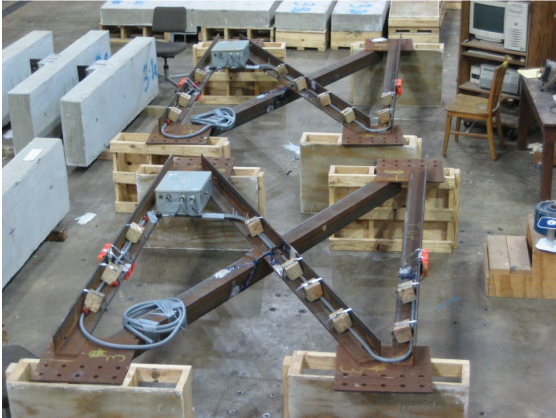
Figure 3.11 Instrumented Cross frames X1 and X2
