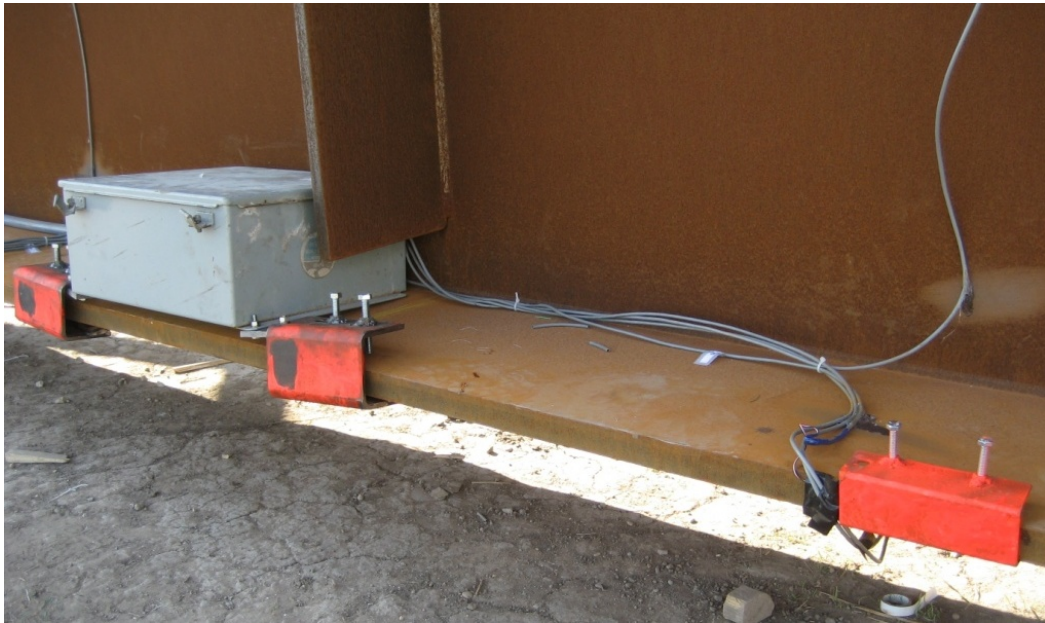
Figure 3.8 Flange Strain gages protected by steel channel caps
