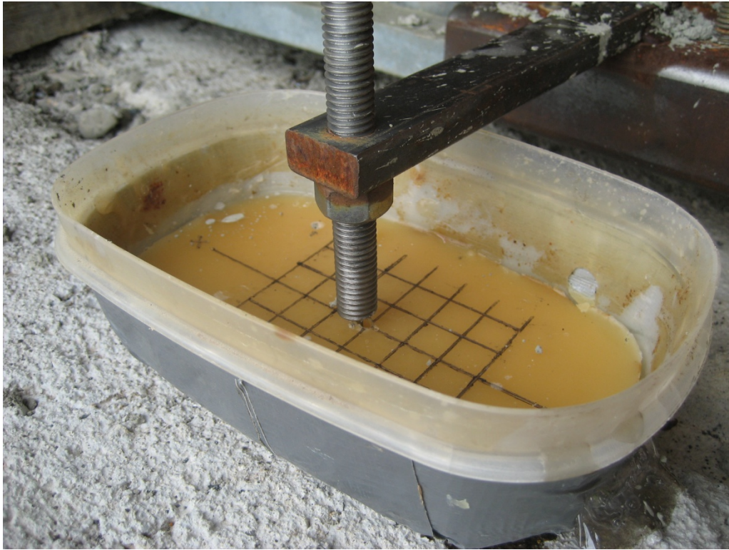
Figure 4.38 Wax Trace Box for Measuring Bearing Movements
