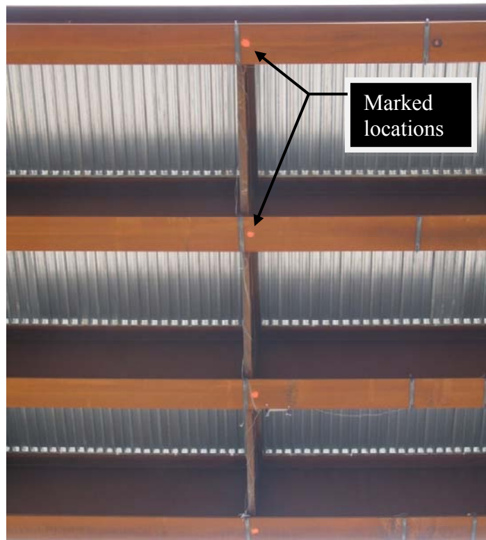
Figure 3.16 Span 14 mid span deflection reading locations
